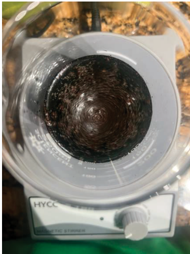
Figure 5 Loose Coffee Grounds in Methylene Blue Solution
